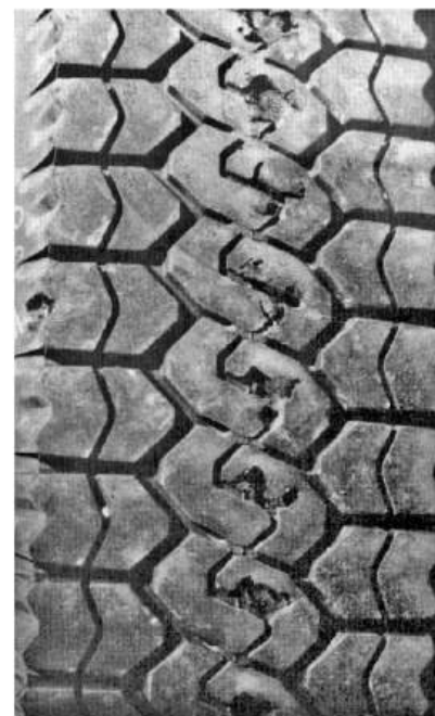
Example of Dyno Damage
